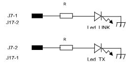
In this case, the led LINK light on for a link down or no link and the led TX light off for a data transmission .
