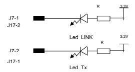
In this case, the led LINK light on for a link up and the led TX light on for a data transmission .
